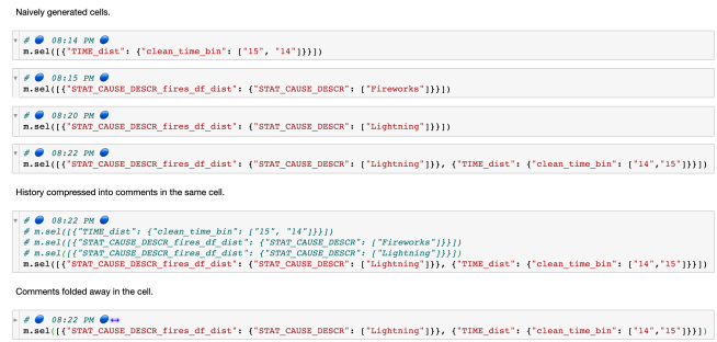
Figure 6. A demonstration of three designs of selection cells. The top four cells represent the result of creating new cells every time there is an interaction. The second last cell represents all four selections, with three commented out. The last cell represents the previous cell folded, and is the design we finalized on for B2.
