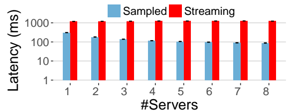
Figure 8: Scalability as we add more servers and increase the dataset proportionally. As before, the ideal scalability corresponds to a constant latency. Note that the Y axis is logarithmic.
