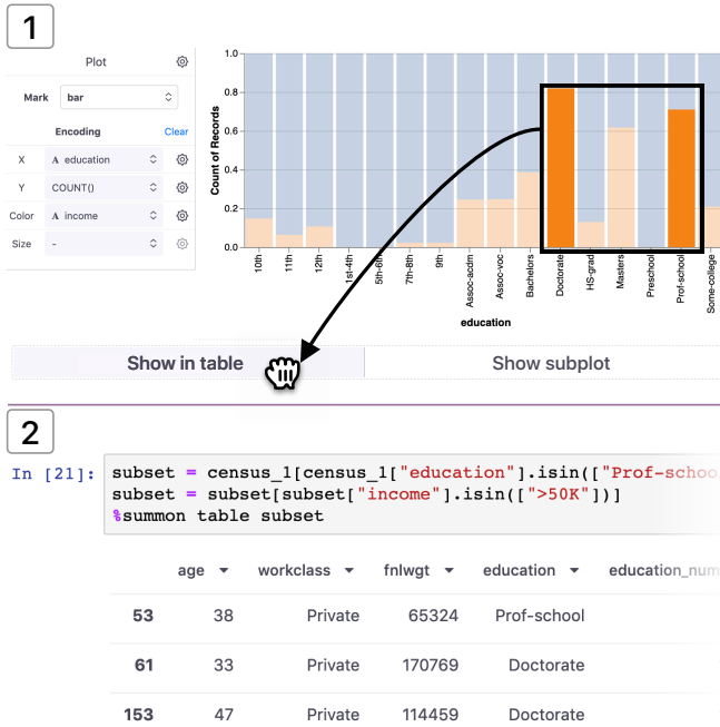
Figure 8: In (1) the user has the plot tool open and has constructed a chart. They select two columns from the chart of interest and begin dragging these columns outside of the chart. As soon as the user starts dragging, an option bin menu appears. The user drags and drops the columns to “Show in table”, and in (2) a new cell is inserted immediately below that displays their selection both in code and in the table tool.
