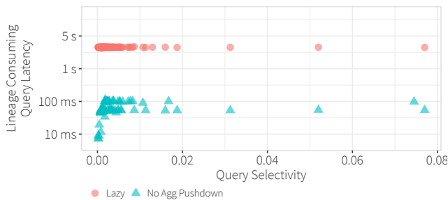
Figure 11: SMOKE-I reduces the lineage consuming query latency by 72.9x on average as compared to LAZY. With aggregation push-down, the latency is \approx 0 ms and we do not plot it.
