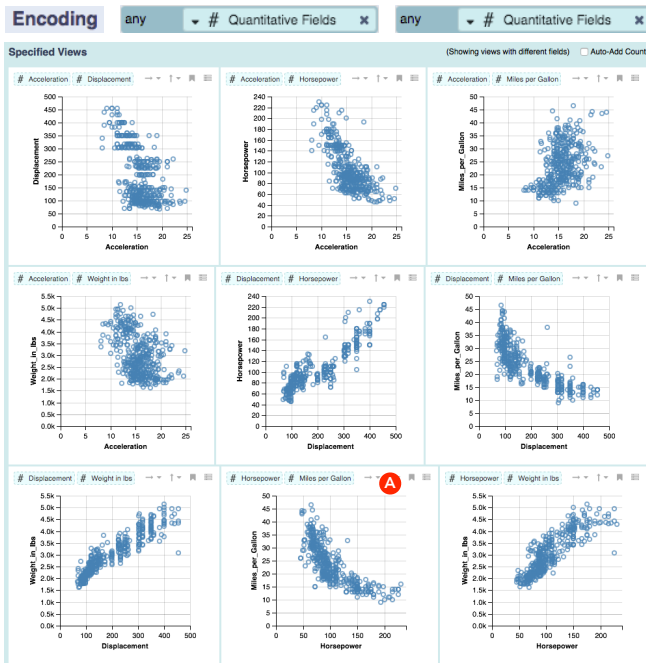
Figure 3. Dropping two quantitative field wildcards onto the wildcard shelves . Voyager 2 automatically chooses encodings, producing scatter-plots that show bivariate relationships between all quantitative fields.
